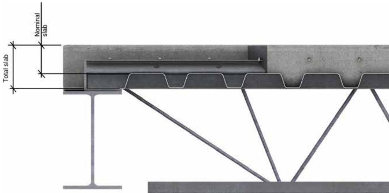
MD2000 slab thickness
