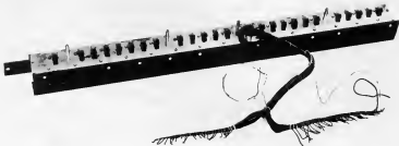
Figure 3-2. Pedal Switch Assembly
