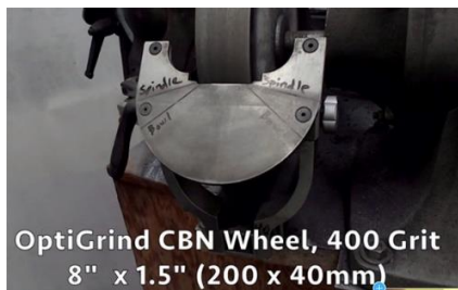
Figure 29 – details of the CBN wheel Figure 30 – demonstration of grind method
