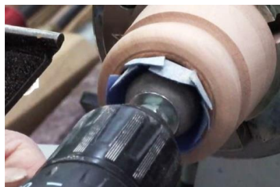
Figure 24 – Power sanding the inside
