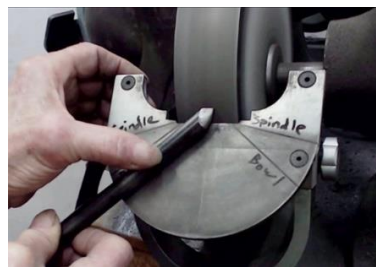
Figure 29 – details of the CBN wheel Figure 30 – demonstration of grind method
