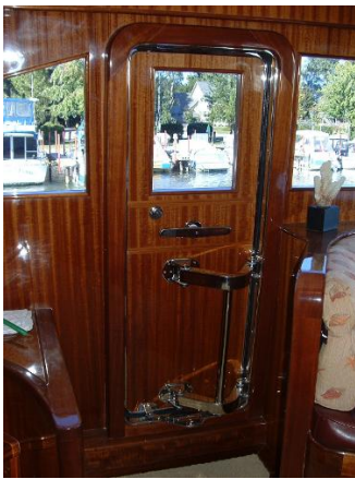
Aircraft-type pilothouse door (starboard)
