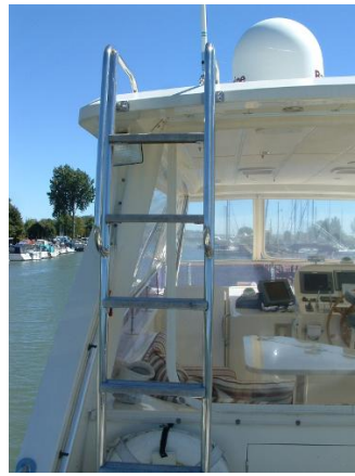
Custom ladder to flying bridge hardtop
