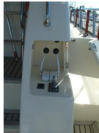
Aft deck control station
