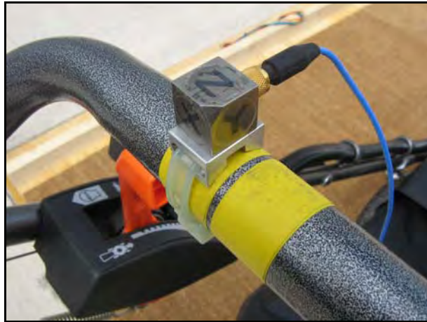
Figure 3 Aluminium block positioned using the cable tie system
