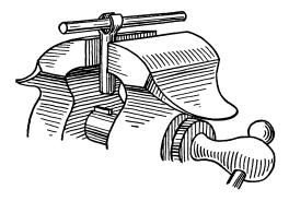
Fig. 29. Scarfs around Small Bars
