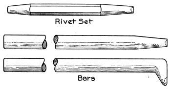
Fig. 62. Tools Used in Riveting
