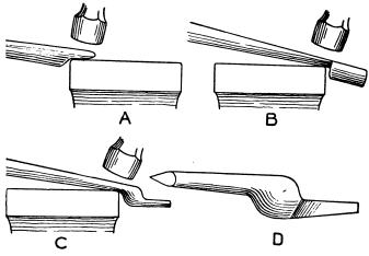
Fig. 5. Method of Forging Tongs
