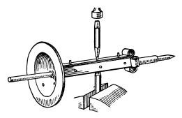
Fig. 120. Riveting the Braces
