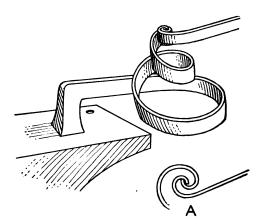
Fig. 67. Former for Scroll-Bending
