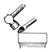
Fig. 24. Drawing to a Point
