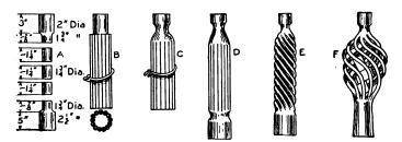
Fig. 55. Method of Forging the Bulb
