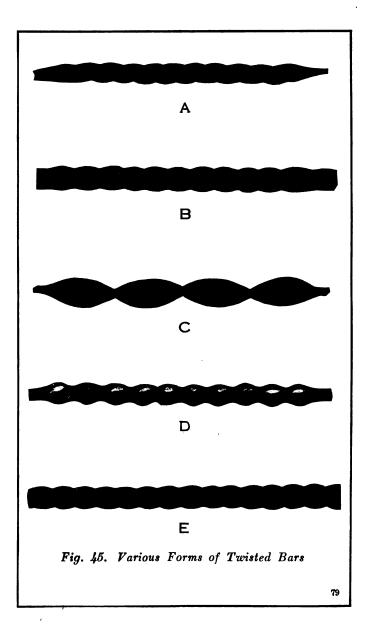
to a uniform heat and twisted. Twists of this kind, with possibly more bars, make very nice handles for pokers and shovels. At B a piece of ½-in. square iron is twisted. At C a piece of
