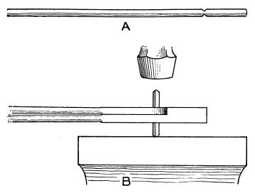
Fig. 7. Making a Rivet for the Tongs
