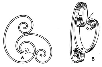
Fig. 75. Method of Riveting Scrollwork
