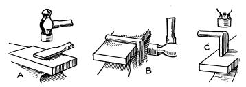
Fig. 107. Making the Handle of a Drawer-Pull
