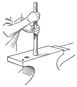
Fig. 15. Upsetting by Ramming
