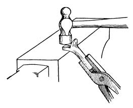
Fig. 27. Forming Scarfs to Fit Bar
