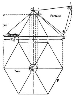
Fig. 117. Drawing for Shade of Electric Lamp
