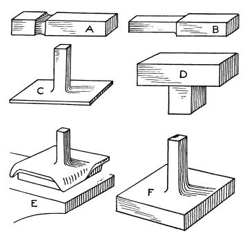
Fig. 79. Method of Forging a Base
