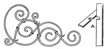
Fig. 64. Riveted Scrollwork
