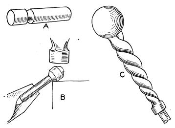
Fig. 59. Working Up a Ball
