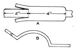
Fig. 42. First Steps in Making an Eye Weld
