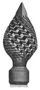
Fig. 56. Bulb Made of Square Rods
