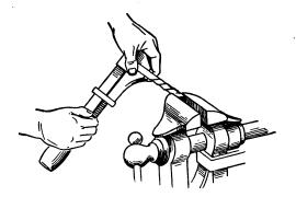
Fig. 44. Twisting a Bar
