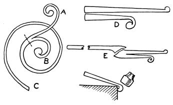
Fig. 76. Method of Welding Scrollwork
