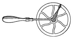
Fig. 21. Traveler, or Tire-Measuring Wheel
