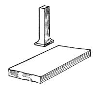
Fig. 35. Stock for a Jump Weld
