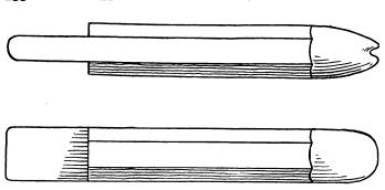
Fig. 86. Sinking-Tool
