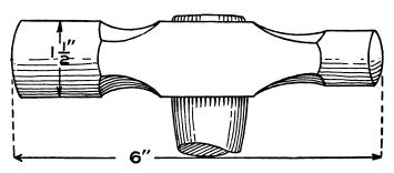
Fig. 100. Hammer Used in Raising
