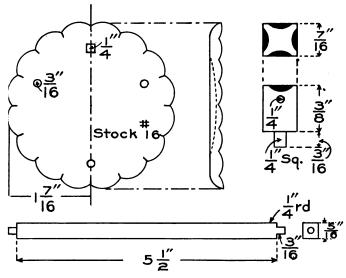
Fig. 109. Drawing for a Pull with Scalloped Plate
