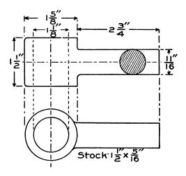
Fig. 41. Welded Eye from Flat Stock
