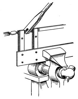
Fig. 48. Twisting Flat Bars
