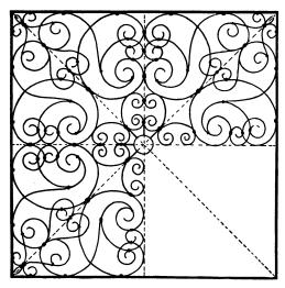
Fig. 3. Laying Out a Design.
