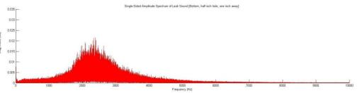
Figure 6 - Filtered amplified leak signal from initial testing
