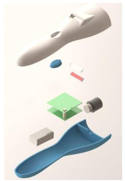
Figure 7 - Solid model of full-production leak detector concept (exploded view)
