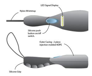
Figure 1 - Conceptual design of leak detector detailing interactive features
