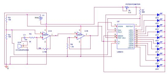
**Figure 4 - Electrical system schematic**
