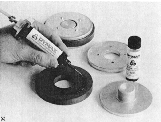
Figure 2 Ferrite assemblies bonded in 10–30 s with aerobic acrylics. (a) Automotive DC motors. (b) Alternators. (c) Loudspeaker. (d) Stepping motors.
