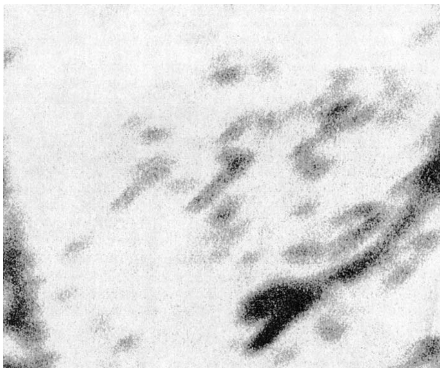
Figure 3 Time-of-Flight SIMS map of the distribution of the intensity of the ion -255 amu originating from stearic acid in lubricant residue at the surface of a cold-rolled steel sample; magnification approximately 500\times ; primary ions ^{69}\text{Ga}^+ of 25 kV.
