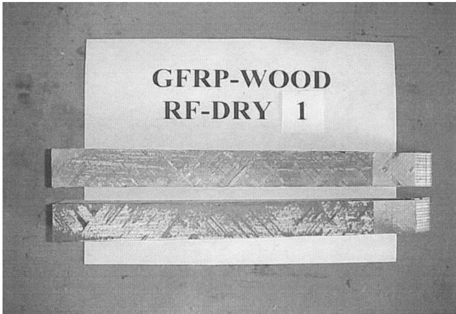
Figure 18 Fracture surfaces of epoxy FRP-wood/RF (specimen 1) under dry conditions.
