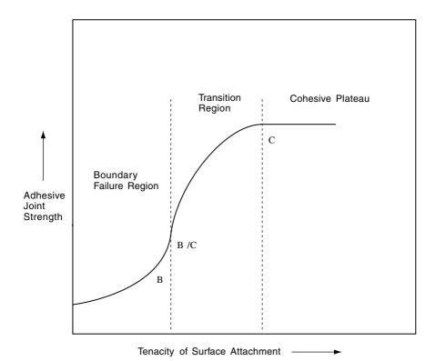
Figure 2.5 Schematic diagram of interfacial states encountered in adhesion. Here B represents boundary failure; C, cohesive failure; and B/C or C/B, mixed failure.<sup>8</sup>
