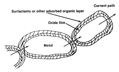
Figure 9.6 Typical current flow path between metal particles in conductive adhesives. Adsorbed organic molecules and oxide films prevent or impede passage of electrons across contact points.<sup>20</sup>
