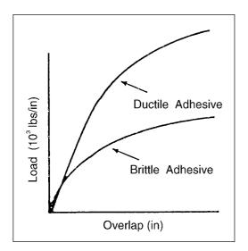
Figure 3.5 Effect of overlap length on failure load using ductile and brittle adhesives.<sup>4</sup>
