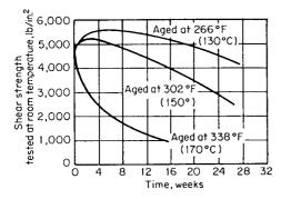
**Figure 17.4** Effect of temperature aging on typical epoxy adhesive in air. Strength measured at room temperature after aging.<sup>6</sup>
