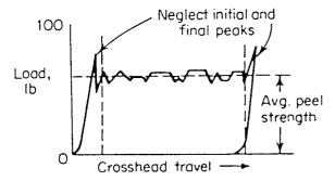
Figure 4.7 Peel test record.4
