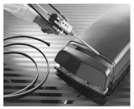
Figure 18.7 Structural bonding of air intake on a tractor. Adhesive is metered and mixed in an on-line static mixing nozzel. (Photo courtesy of Sealant Equipment and Engineering, Inc.)
