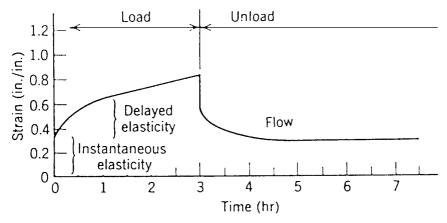
Figure 4.22 Typical creep curve for sealant.<sup>20</sup>
