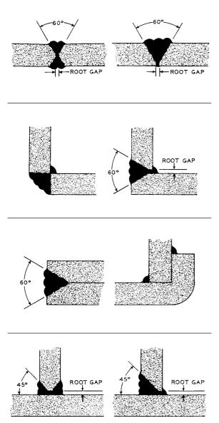
Figure 15.4 Conventional hot gas welding joint designs. 10
