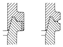
Circular parts can be joined more effectively with tongue-in-groove joints which retain most of the melt and create a joint of high integrity.
