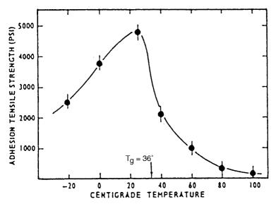
Figure 2.21 Adhesive joint strength of a carboxylic acid containing acrylic terpolymer to aluminum as a function of temperature.<sup>8</sup>
