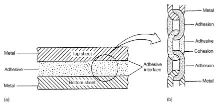
**Figure 6.1** In an ideal joint the substrate should be the weakest link. The adhesive joint (a) can be divided into at least five regions that are similar to the links (b) in a chain.<sup>1</sup>
