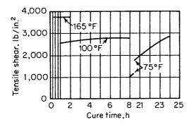
Figure 10.1 Characteristics of a particular epoxy adhesive under different cure time and temperature relationships.<sup>1</sup>
