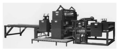
Figure 18.12 Hot melt laminating system can produce 66 inch wide product. (Photo courtesy of Harlan Machinery Company.)
