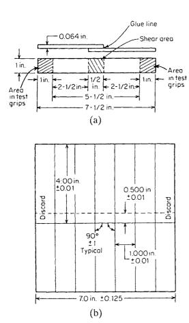
**Figure 4.4** Standard lap shear test specimen design: (a) form and dimensions of lap shear specimen; (b) standard test panel of five lap shear specimens. From ASTM D 1002
