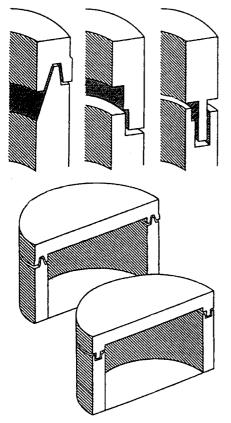
Figure 15.7 Common joints used in the spin welding process.  $^{18}$
