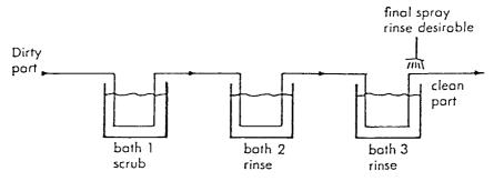
Figure 6.6 Three bath method of solvent immersion cleaning.<sup>20</sup>
