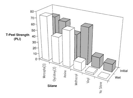
Isocyanate Terminated Urethane, Adhesion to Aluminum
