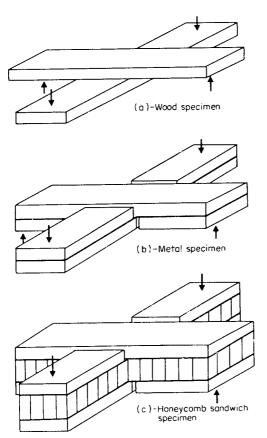
Figure 4.3 Cross-lap tension test specimen.<sup>4</sup>
