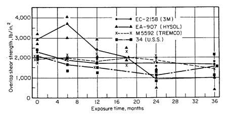
Figure 17.12 Effect of outdoor weathering on typical aluminum joints made with four different two part epoxies cured at room temperature.<sup>30</sup>
