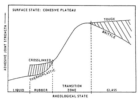
Figure 2.22 Schematic diagram of the effect of the rheological state on adhesive lap shear and tensile joint strengths.<sup>8</sup>
