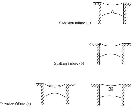
Figure 2.16 Cohesion (a), spalling (b), and intrusion failure (c) modes of a sealant joint.<sup>22</sup>
