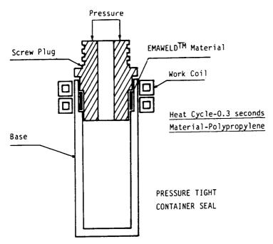
Figure 15.6 Schematic of induction welded plastic nozzle; adhesive is supplied by  ${\it Emaweld.}^{15}$
