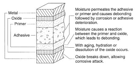
Figure 2.23 Examples of weak boundary layers.<sup>24</sup>
