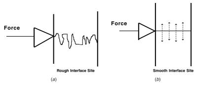
**Figure 2.8** Schematics showing (a) tortuous interface between two adhering materials with rough surfaces and (b) two adherends with smooth surfaces. Note that in (a) the applied force cannot cleanly follow the path between the two adherends and as excursions are made energy is dissipated. <sup>10</sup>
