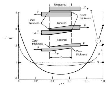
Figure 3.11 Shear stress distribution in bonded joints: untapered (1), tapered and finite thickness (2), and tapered and zero thickness (3).
