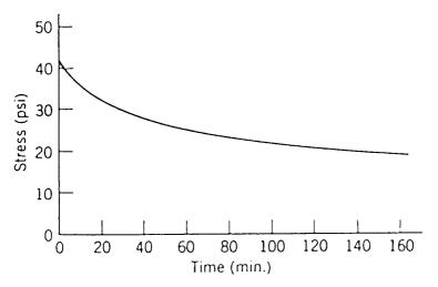
Figure 4.21 Typical stress relaxation curve for sealant.<sup>20</sup>
