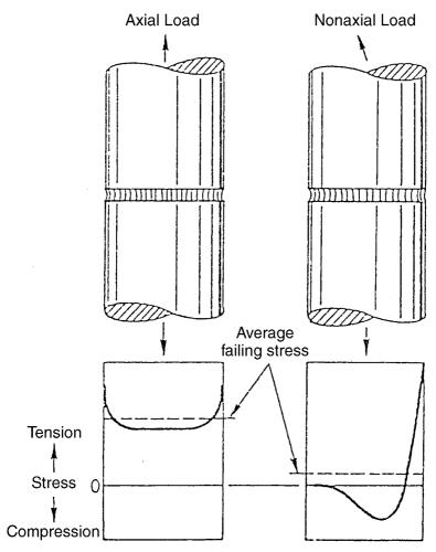
Figure 3.2 Stress distribution in a butt joint under axial and non-axial loading.<sup>1</sup>
