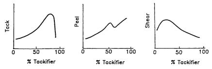
Figure 9.2 Dependence of tack, peel, and shear on resin/tackifier ratio.4
