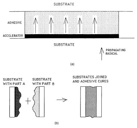
Figure 8.3 Reactive acrylic adhesives can cure via an "accelerator cure" mechanism (a) or by a "honeymoon cure" mechanism (b).
