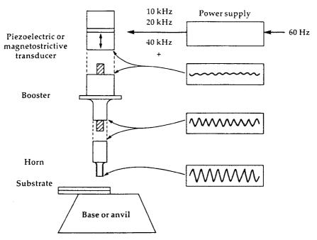
Figure 15.8 Equipment used in a standard ultrasonic welding process.<sup>20</sup>
