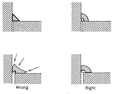
Figure 3.30 Design of corner sealant joints.<sup>14</sup>
