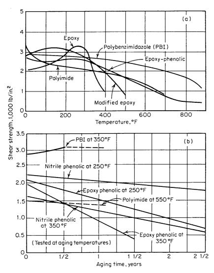
Figure 17.3 Comparison of (a) heat resistance and (b) thermal aging of several high temperature structural adhesives.<sup>5</sup>
