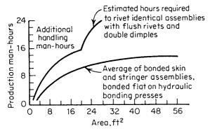
Figure 1.8 The economy of metal-to-metal bonding compared with conventional riveted structure.<sup>9</sup>
