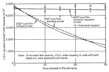
Figure 7.2 Effect of primer on lap-shear strength of aluminum joints exposed to 5 percent salt spray.<sup>2</sup>
