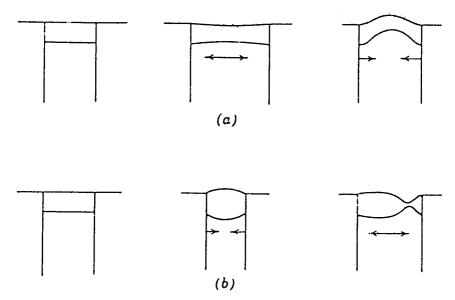
Figure 2.17 Change in sealant shape due to flow. (a) Viscous tension-compression effect. (b) Viscous compression-tension effect. (a) Viscous tension-compression effect.
