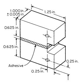
Figure 4.14 Cleavage test specimen. [From ASTM D 1062]
