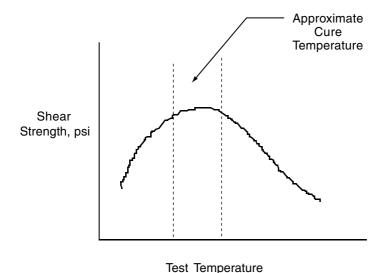
**Figure 2.14** Plot of the strength of an aluminum joint (bonded with an elevated temperature curing epoxy adhesive) as a function of test temperature.
