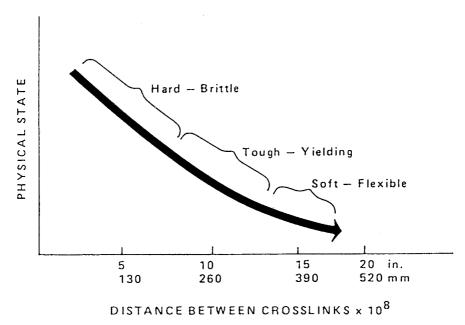
Figure 2.19 Effect of crosslink density on the physical state of epoxy resins.<sup>21</sup>
