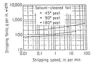
Figure 4.8 Peel strength of 3 mil aluminum foil bonded with DETA cured DGEBA epoxy adhesive.<sup>9</sup>
