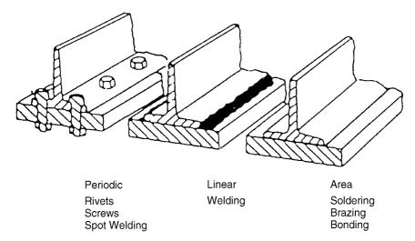
Figure 1.5 Periodic, linear, and area attachment systems.<sup>5</sup>
