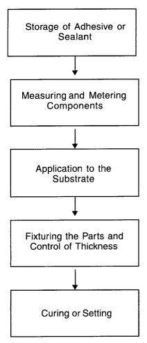
Figure 18.1 Major processes in producing adhesive or sealant joints.
