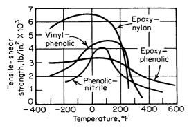
Figure 10.4 The effect of temperature on the tensile shear strength of modified epoxy adhesives (substrate is aluminum).<sup>3</sup>
