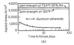
**Figure 17.11** Time to failure vs. stress for two adhesives in a warm, high humidity environment. (a) One part, heat cured modified epoxy adhesive. (b) Flexibilized amine cured epoxy adhesive. <sup>27</sup>
