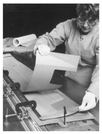
Figure 18.11 AF-32 nitrile-phenolic adhesive film bonds doubler stacks in aerospace application. Adhesive provides vibration damping. (Photo courtesy of 3M Company.)
