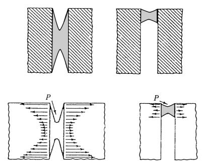
Figure 3.24 Comparisons of maximum strains (left) for a 2 inch deep seal; extension of joint 100%, sealant strain 550%; and (right) for a ¼ inch deep seal; extension of joint 100%, sealant strain 160%. 14
