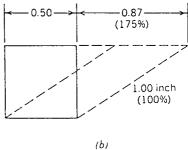
Figure 3.27 Movements in lap shear joints. Original sealant dimensions are  $\frac{1}{2} \times \frac{1}{2}$  inches. (a) Displacement of 0.56 inches with sealant only extended 50%, using a  $\pm 50\%$  capacity sealant (medium modulus). (b) Displacement of 0.87 inches with sealant only extended 100%, using sealant with  $\pm 100\%$  extension capability (low modulus). (14)
