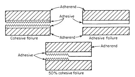
Figure 1.1 Examples of cohesive and adhesive failure.
