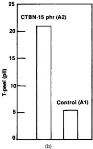
Figure 9.3 Lap shear (a) and peel strength (b) comparison of control epoxy adhesive formulation and one containing 15 phr CTBN elastomer.<sup>11</sup>
