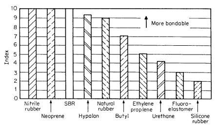
Figure 16.7 Bondability index of common and specialty elastomers.<sup>72</sup>
