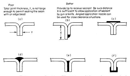
**Figure 14.6** Various seam sealing joints. Edge (a) is not thick enough to support bead. Lip joint (b) provides receptacle for sealant. Seam can be inside sealed by tape (c), putty (d), or sandwich sealed with putty or anaerobic (e), tape can also be used on the outside of seam (f).
