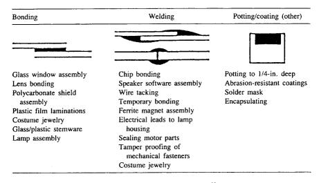
Figure 8.4 Bonding categories using UV aerobic adhesives. 10
