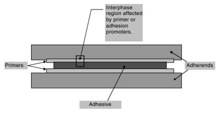
**Figure 7.1** Primers and adhesion promoters provide a stronger interphase region having improved adhesion and permanence.
