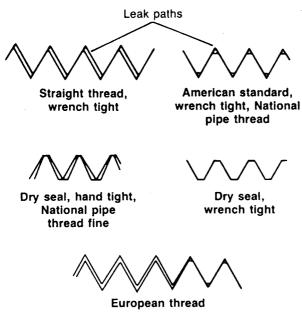
Figure 14.7 Thread designs for threaded fittings.<sup>4</sup>
