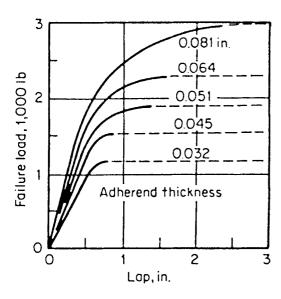
**Figure 3.8** Interrelation of failure loads, depth of lap, and adherend thickness for lap joints with a specific adhesive and adherend <sup>7</sup>
