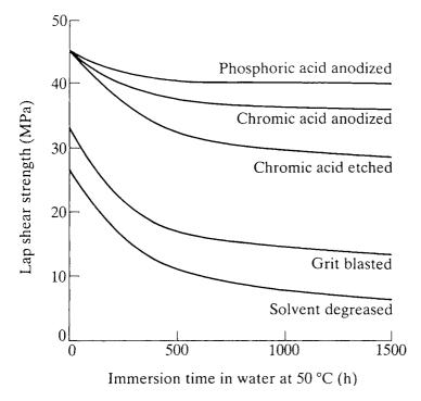
Figure 6.4 Effect of surface pretreatments on the performance of aluminum joints bonded with a toughened epoxy adhesive and subjected to aging in water at  $50^{\circ}$ C.
