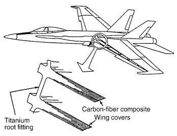
Figure 16.5 F-18 wing to fuselage attachment.<sup>67</sup>
