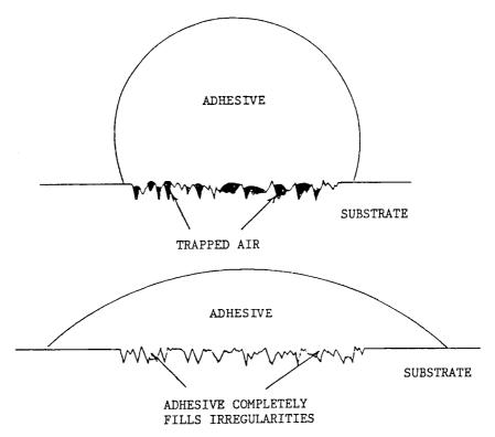
Figure 1.10 Illustration of poor (top) and good (bottom) wetting by an adhesive spreading over a surface.
