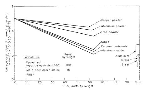
Figure 9.4 The coefficients of thermal expansion of filled epoxy resins compared with those of common metals. $^{13}$
