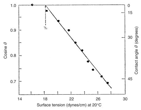
Figure 2.3 Zisman plot for determining critical surface tension of polytetrafluoroethylene. Test liquids are n-alkanes.<sup>5</sup>
