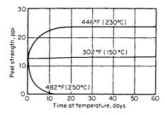
Figure 10.9 Peel strength of RTV silicone rubber bonded to aluminum as a function of heat aging.<sup>37</sup>
