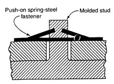
Figure 15.18 Push-on spring steel fasteners.<sup>29</sup>
