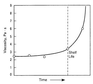
Figure 18.2 Increase in viscosity of a paste adhesive as a function of time at room temperature.<sup>3</sup>
