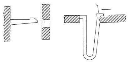
Figure 15.20 Snap fitting cantilevered arms.<sup>29</sup>
