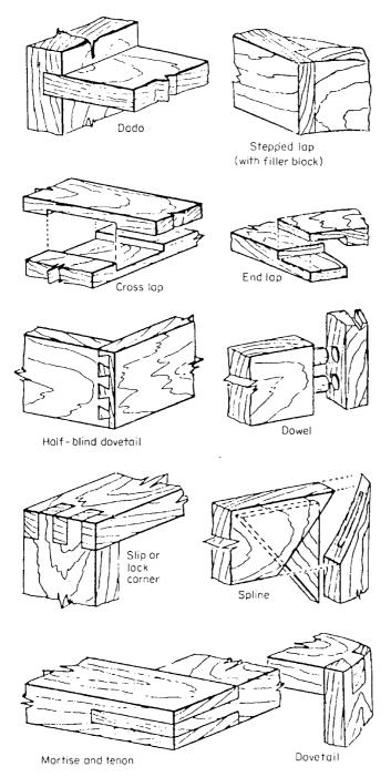
Figure 3.21 Construction adhesive joints for wood.<sup>1</sup>
