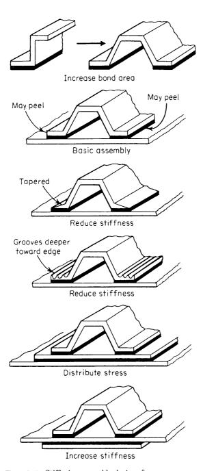
Figure 3.15 Stiffening assembly designs. $^9$
