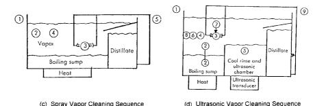
**Figure 6.7** Representative methods of vapor degreasing: (a) straight vapor cleaning, (b) immersion vapor cleaning, (c) spray vapor cleaning, and (d) ultrasonic vapor cleaning. Numbers represent the sequence in the processing steps.<sup>20</sup>
