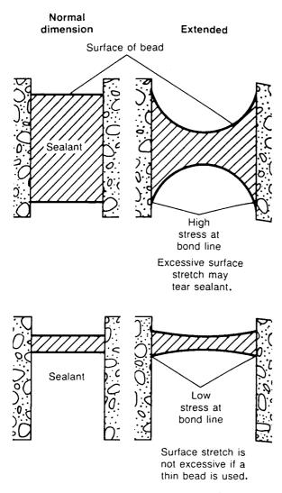
Figure 14.2 Sealant bead thickness and stress.<sup>2</sup>
