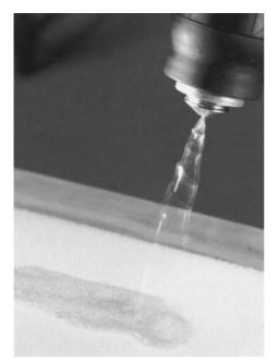
Figure 18.9 Hot melt adhesives can be applied by spray application for fast bonding of most foams, plastics, fabrics, particle board, and light gauge metals. (Photo courtesy of 3M Company.)
