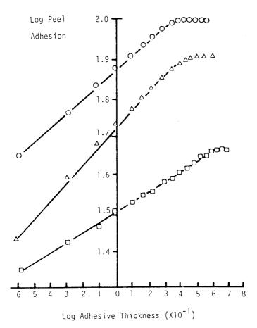
Figure 4.13 Comparison of peel force with adhesive thickness (0.5 mil polyester film used as backing in all tests).
