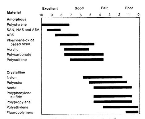
Figure 15.10 Ultrasonic weldability index for common thermoplastics.<sup>22</sup>
