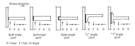
Figure 3.17 Angle joint designs. 9
