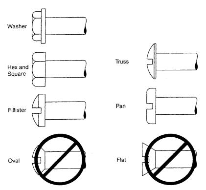
Figure 15.16 Common head systems of screws and bolts. Flat underside of head is preferred.  $^{29}$
