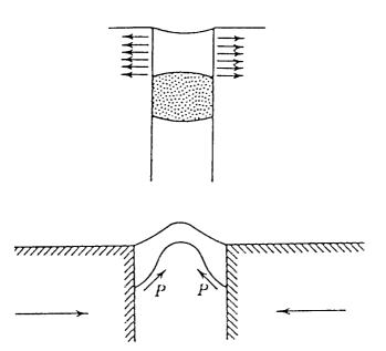
Figure 3.26 Tooled sealant showing (top) uniform substrate stress and (bottom) under compression if the sealant is too thin. 14
