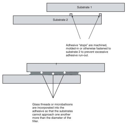
**Figure 11.4** Adhesive starvation in a joint can be prevented by incorporating shims (top) in the substrate itself, or (bottom) directly within the adhesive.
