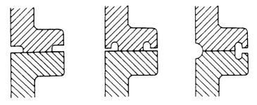
Unless the parts have thick walls it is necessary to form a flange for the butt weld. In practice melt traps are usually formed so that the molten resin does not create a flashing.
