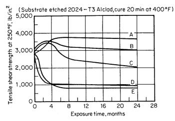
Figure 17.13 Effect of immersion in various chemical environments on a one part heat curing epoxy adhesive (EA929, Hysol Corp.). (a) gasoline at 75°F, (b) gear oil at 250°F, (c) distilled water at 75°F, (d) tapwater at 212°F, (e) 38% Shellzone at 250°F. $^{35}$
