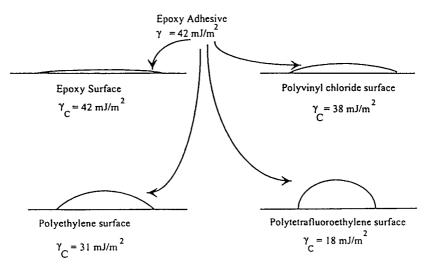
**Figure 2.7** Contact angle of an uncured epoxy adhesive on four surfaces of varying critical surface tension. Note that as the critical surface tension of the surfaces decrease, the contact angle increases indicating less wetting of the surface by the epoxy.<sup>10</sup>
