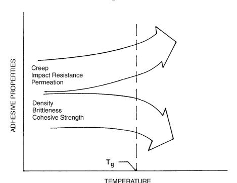
Figure 2.18 General trends of some adhesive properties related to temperature or molecular mobility. The sharp change at the  $T_{\rm g}$  reflects the abrupt increase in molecular motion.  $^{21}$
