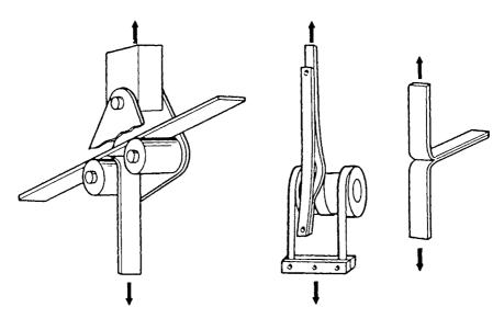
$\textbf{Figure 4.6} \quad \text{Common types of adhesive peel tests: (left) floating roller peel, (center) climbing drum peel, (right) t-peel. \\ ^6$
