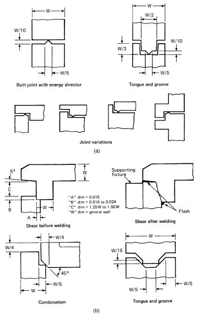
Figure 15.11 Ultrasonic welding joints for (a) amorphous and (b) crystalline polymeric materials.  $^{23}$
