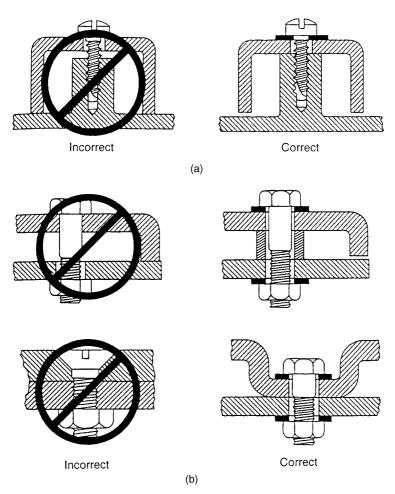
Figure 15.15 Mechanical fastening with self taping screws (a) and with bolts, nuts, and washers (b).<sup>29</sup>
