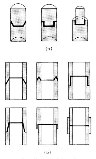
Figure 3.16 Designs for rod and tube joints. (a) Three designs for round bars. (b) Six designs for cylinders or tubes. 10
