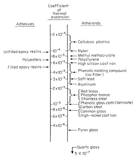
Figure 2.12 Thermal expansion coefficients of common materials. 18
