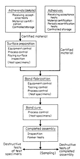
Figure 5.1 Flow chart of a quality control system for adhesive bonding.<sup>1</sup>
