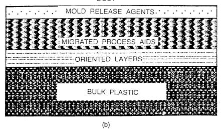
Figure 6.2 Schematic representation of metal (a) and polymer (b) substrate surface regions.
