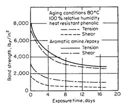
Figure 17.9 Effect of humidity on adhesion of two structural adhesives to stainless steel.<sup>21</sup>
