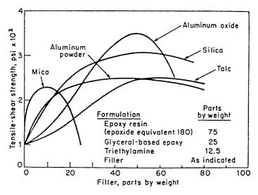
Figure 9.5 The effect of mineral extenders on the tensile shear strength of epoxy adhesives (the substrate is aluminum).<sup>14</sup>
