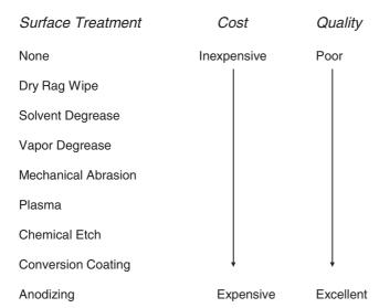
**Figure 6.5** The objective of surface preparation is to provide a consistent, reproducible adherend surface that when bonded meets the strength and durability required for the application.
