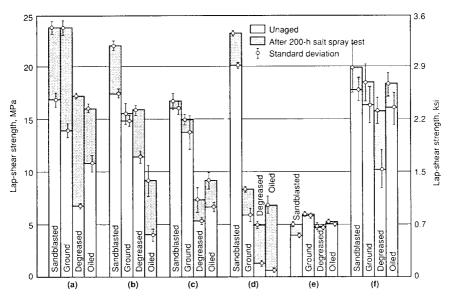
Figure 16.3 Shear strength of mild steel joints. (a) Two part cured epoxy. (b) Two part acrylic. (c) Anaerobic acrylic. (d) Cyanoacrylate. (e) PVC plastisol. (f) One part heat cured epoxy.  $^{27}$
