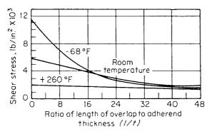
**Figure 3.6** The effect of ratio of length of overlap to adherend thickness (l/t) on adhesive strength at three test temperatures for aluminum joints bonded with a nitrile rubber adhesive.<sup>5</sup>
