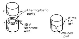
Figure 15.5 Resistance wire welding of thermoplastic joints.  $^{11}$
