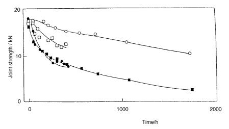
Figure 6.9 Effect of high humidity (97% relative humidity at 43°C) on the strength of aluminum joints bonded with an epoxy-polyamide adhesive. Surface treatments are (○) chromic–sulfuric acid etch, (□) alkaline etch, (●) solvent degrease, and (■) phosphoric acid anodize. $^{30}$
