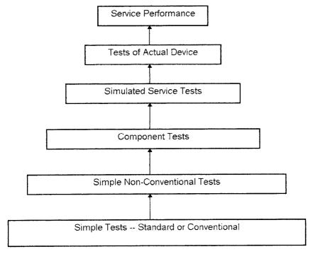
Figure 4.23 Testing hierarchy as illustrated by the "Mathes ladder". <sup>23</sup>
