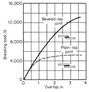
Figure 3.12 The effect of beveled and plain lap-joint design on breaking load.  $^{\rm 8}$
