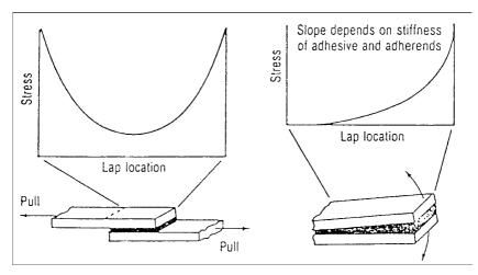
Figure 3.3 Stress distribution on an adhesive when stressed in (left) shear and (right) peel or cleavage. $^2$
