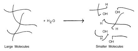
Figure 17.6 The degradation of polymer chains by reaction with water hydrolysis. 18
