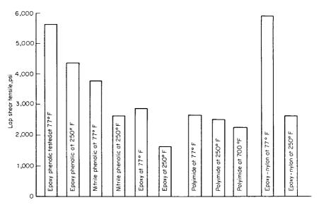
Figure 16.2 Bond strength for beryllium to beryllium joints using various adhesives and a sulfuric acid—sodium dichromate etch.<sup>17</sup>
