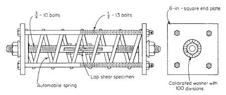
Figure 4.16 Compressive spring with tension creep-shear specimen.<sup>4</sup>
