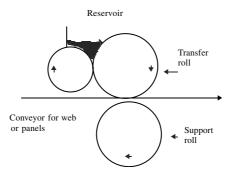
Figure 18.10 Methods of machine application of adhesive coatings.  $^{10}$
