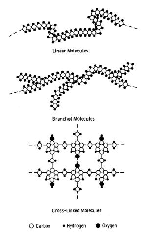
Figure 8.1 Some possible molecular structures in polymeric resins used as adhesives.<sup>1</sup>
