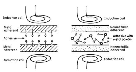
**Figure 18.13** Left—induction heating metal parts heat adhesive by conduction. Right—Parts not heated by induced electric currents are bonded with an adhesive that can be heated because it contains metal particles. <sup>14</sup>
