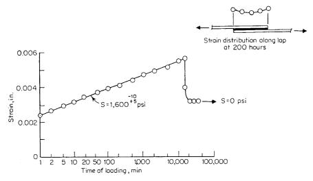
Figure 4.17 Typical creep-time curve for a lap shear adhesive joint bonded with a visco-elastic adhesive.<sup>4</sup>
