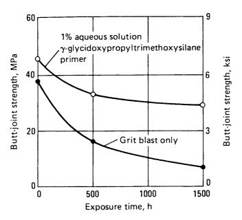
Figure 7.4 Effect of silane adhesion promoter on the durability of a mild steel joint bonded with epoxy adhesives.<sup>32</sup>
