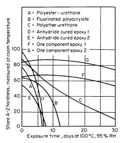
Figure 17.7 Hydrolytic stability of potting compounds. Materials showing rapid loss of hardness in this test soften similarly after 2–4 years in high temperature, high humidity climate zones.<sup>19</sup>
