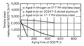
Figure 17.1 The effect of  $500^{\circ}F$  aging in air and nitrogen on an epoxy phenolic adhesive (HT-424).<sup>3</sup>
