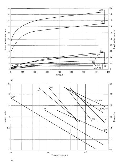
Figure 16.4 Typical bond durability data for Ti-6Al-4V adherends bonded with an epoxy adhesive and aging at  $60^{\circ}$ C and 100% relative humidity. (a) Crack propagation versus time for the wedge crack propagation test. (b) Applied stress versus time to failure for the lap shear geometry. PF—phosphate fluoride; MPF—modified phosphate fluoride; DP—PasaJell 109 dry hone; LP—Pasa Jell 107 liquid hone; CAA5—5% solution; CAA10—10% solution; TU—Turco 5578 etch; DA-Dapcotreat. 38
