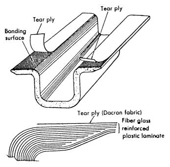
Figure 6.12 Structural reinforced plastic laminate with tear ply to produce fresh bonding surface.<sup>20</sup>
