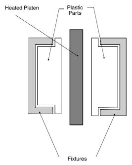
Figure 15.1 In direct hot plate welding, two fixtures press components into a hot moving platen, causing the plastic to melt at the interface.
