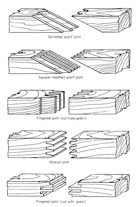
Figure 3.20 End joints for wood.1
