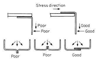
Figure 3.19 Joint designs for flexible substrates.9
