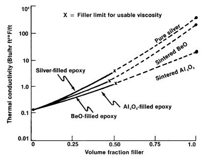
Figure 9.7 Thermal conductivity increases as filler loading increases, but loading is limited by mixture viscosity to a maximum of 40-50% by volume.<sup>20</sup>
