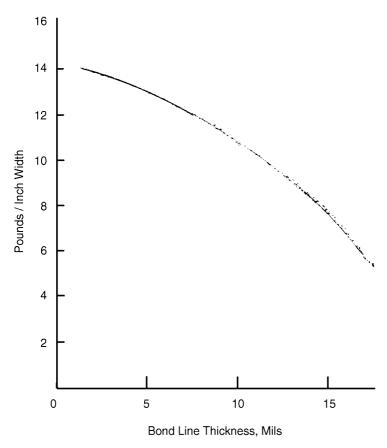
Figure 4.9 Effect of adhesive thickness on peel resistance of Resiweld 7007 epoxy adhesive.  $^{7}$
