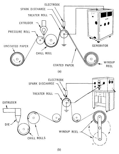
Figure 6.10 Basic arrangements for corona surface treating of (a) plastic coated paper and (b) plastic film.
