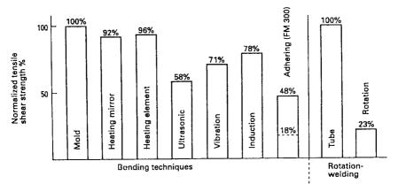
Figure 16.6 Comparison of the normalized tensile yield strength of thermoplastic advanced composite bonds produced by selected techniques.<sup>68</sup>
