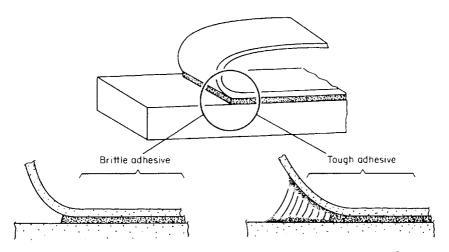
Figure 3.4 Tough, flexible adhesives distribute peel stress over a larger area.<sup>3</sup>
