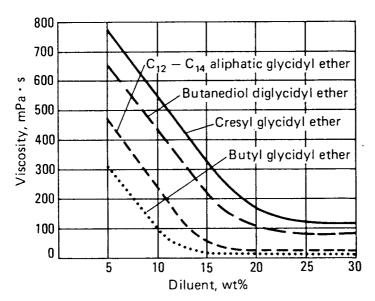
Figure 9.1 Reduction of diglycidyl ether of bisphenol A (DGEPA) epoxy resin by reactive diluents.  $^{\rm l}$
