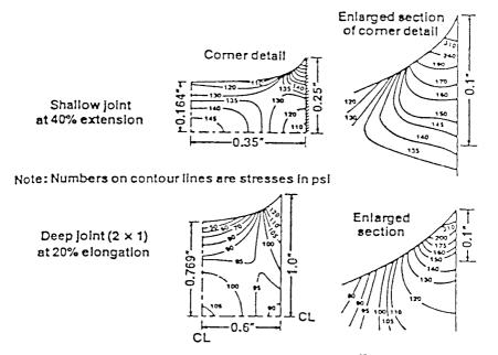
Figure 3.23 Unequal stress distributions in sealant butt joints. 13
