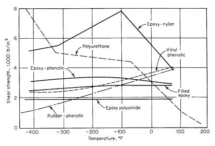
Figure 17.5 Properties of cryogenic structural adhesives systems.<sup>5</sup>
