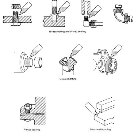
Figure 8.6 Anaerobic adhesive applications. 11
