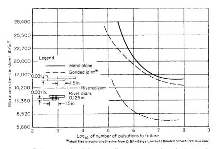
Figure 1.7 Fatigue strengths of aluminum-alloy specimens under pulsating tensile load.<sup>8</sup>
