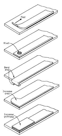
**Figure 3.14** Minimizing peel in adhesive joints.<sup>9</sup>
