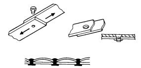
When joining a material with mechanical fasteners, holes must be drilled through the assembly. These holes weaken the material and allow concentration of stress.
