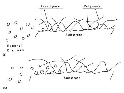
**Figure 2.15** Competition between an adhesive and other chemicals for surface sites leading to displacement of the adhesive from the surface. (a) Adhesive adsorbed at surface sites. (b) Adhesive displaced from surface sites. a1
