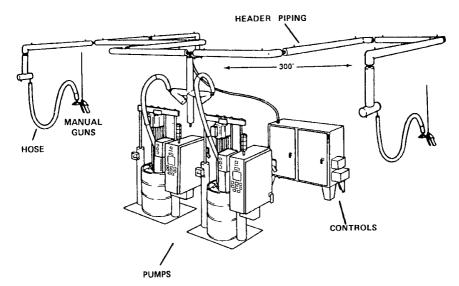
Figure 18.8 Modular header system.<sup>6</sup>
