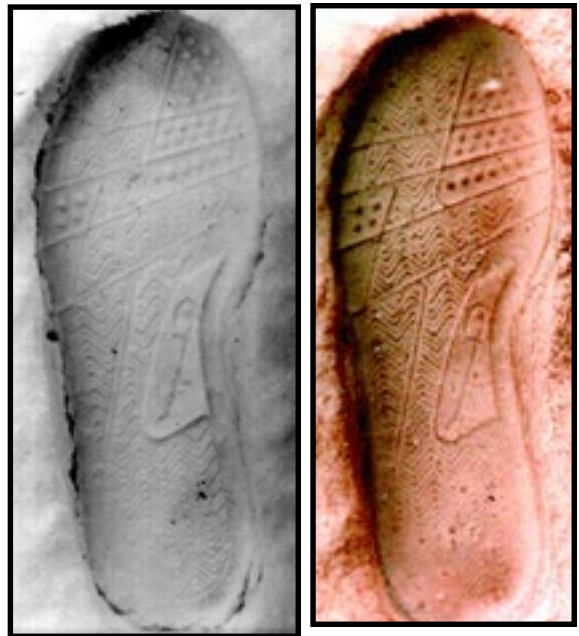
Shoe impressions in snow: Shoeprint examiners have difficulty analyzing low-contrast photographs such as the one on the left. The shoeprint on the right has been sprayed with colored paint to increase contrast, which produces a more detailed photograph.
