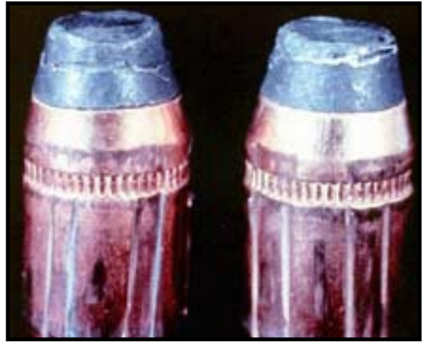
Rifling characteristics on fired bullets.
