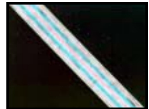
Polarizing microscope image of a nylon fiber.
