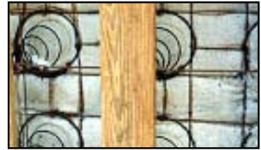
Thermally damaged box springs.
