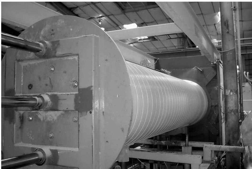
Fig. 4.5 Sewer pipe manufactured to ASTM F1803 undergoing required air test.
