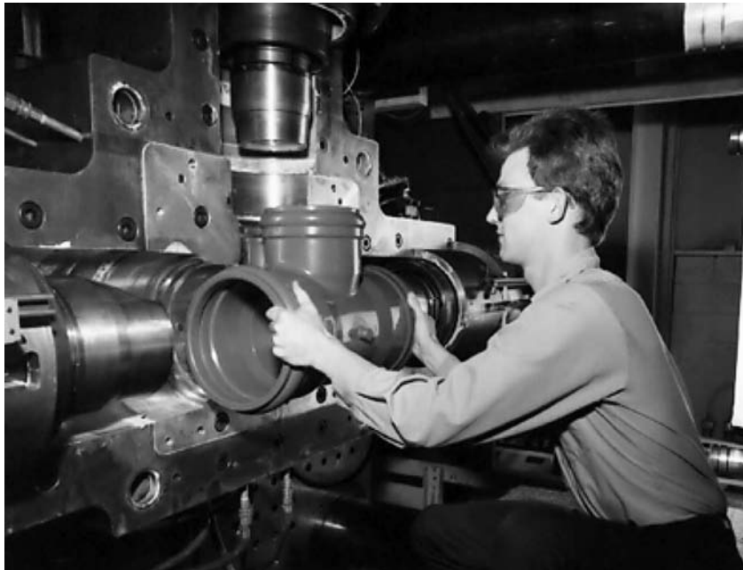
Fig. 4.7 The operator is demonstrating how a PVC Pressure Class 235 Tee would be positioned in the injection molding machine.
