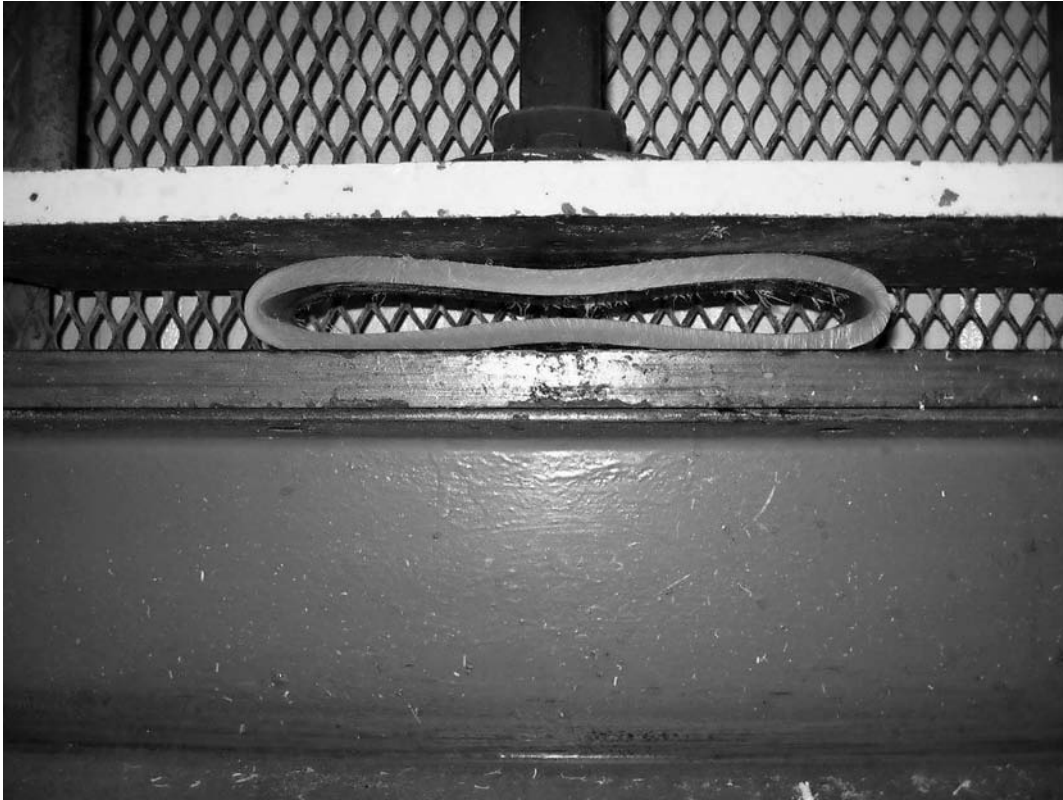
Fig. 4.11 PVC pipe undergoing a flattening test.
