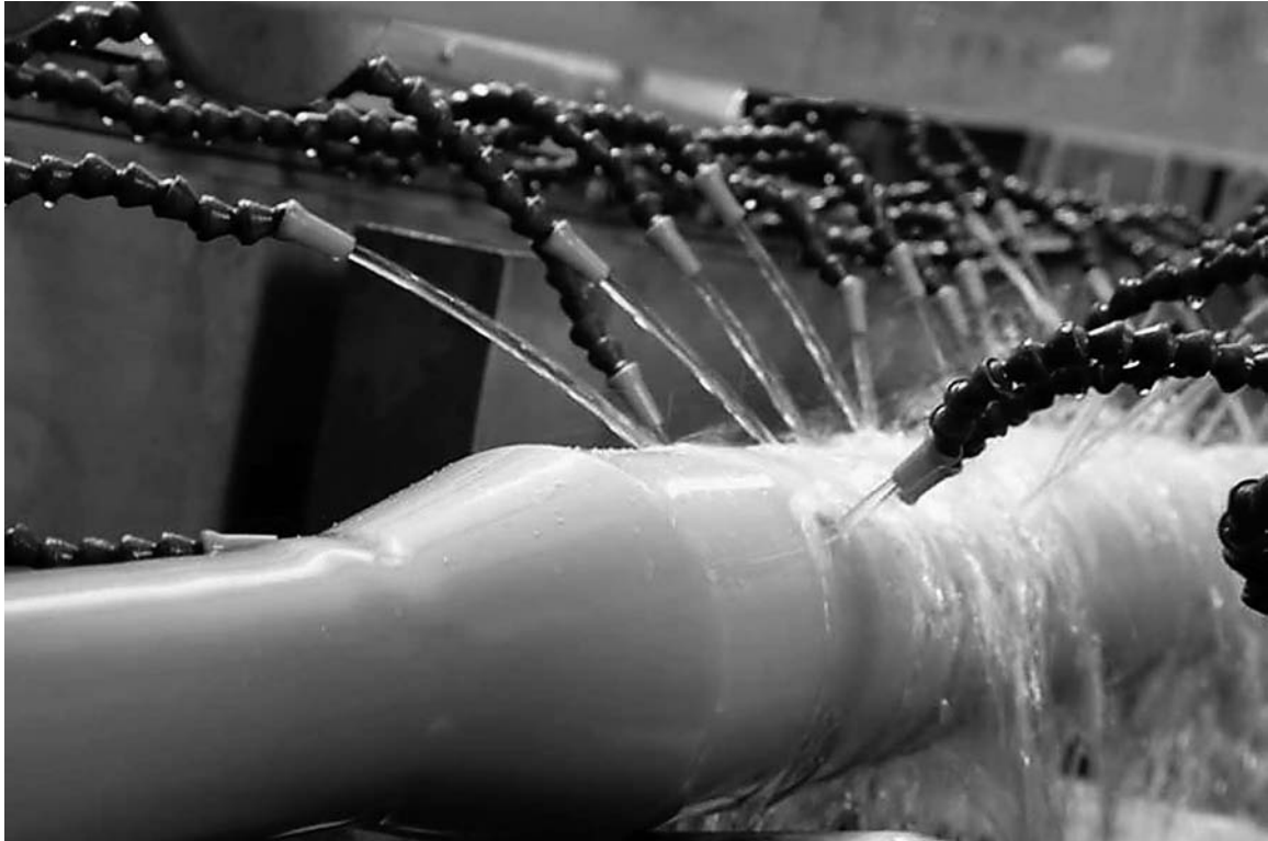
Fig. 14.1 PVCO – Continuous process.
