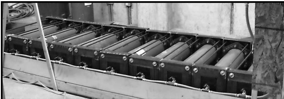
Fig. 5.3 Apparatus for collecting stress-rupture data.
