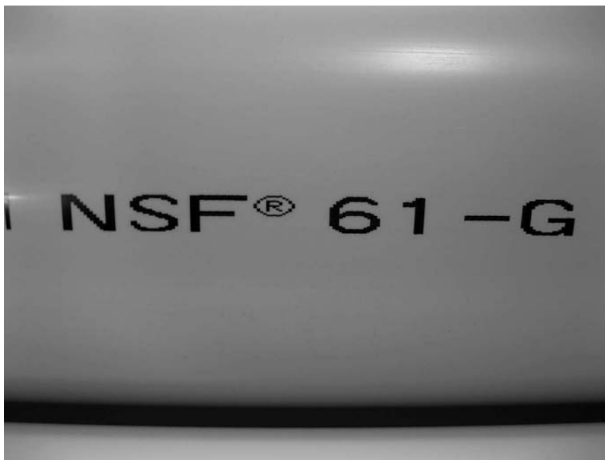
Fig. 1.3 PVC pipe for potable water service, marked to show NSF Standard 61 certification.
