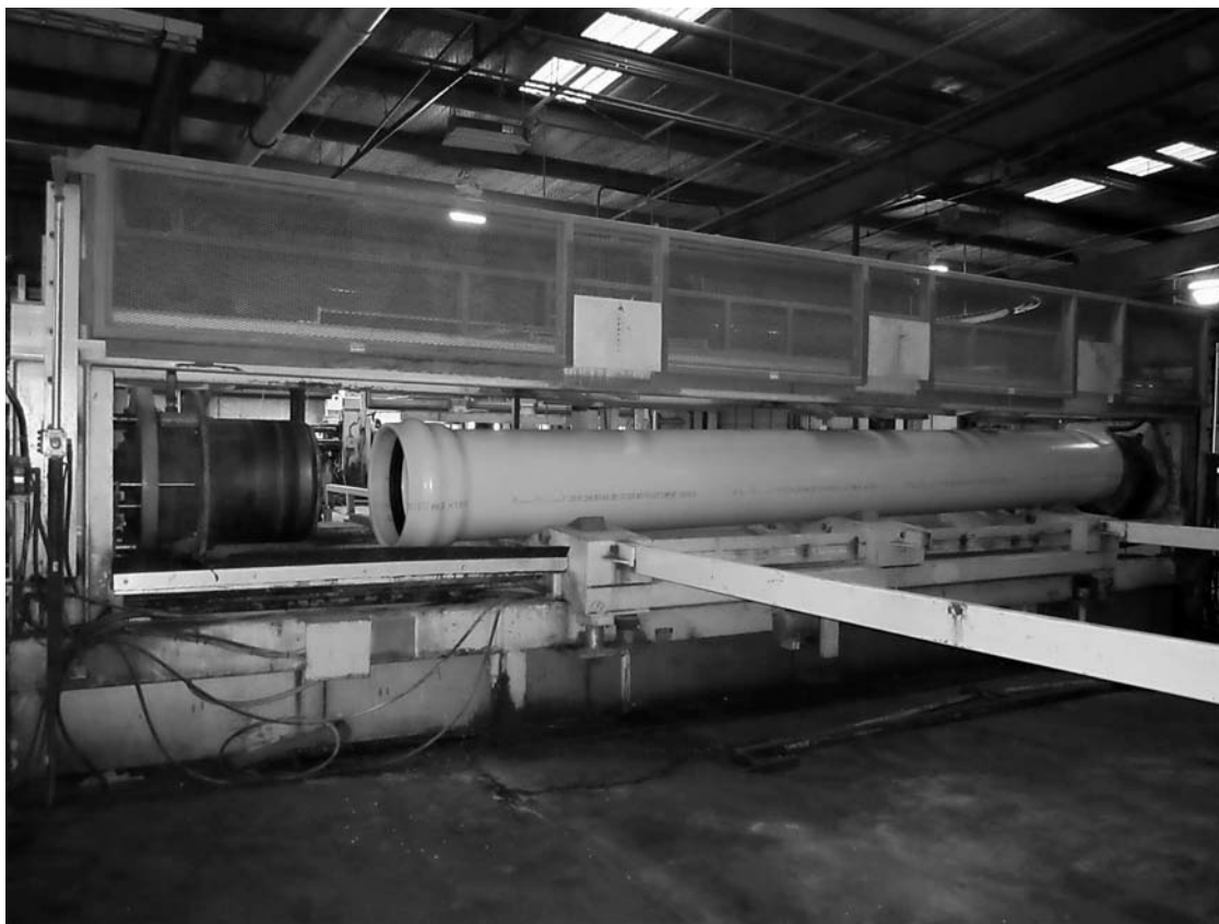
Fig. 4.12 Hydrostatic proof test of PVC pressure pipe.
