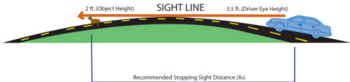
Figure 4.12. Heights Pertaining to Stopping Sight Distance
