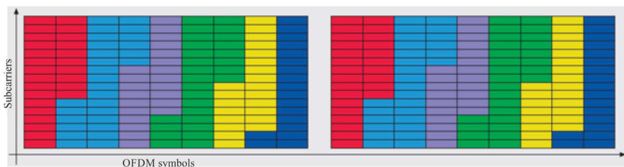
FIGURE 9.46 Different PLPs occupying different slices of individual modulation, code rate and time interleaving, two frames are shown
