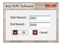
You can specify the record number by typing in the window. **Note:** the start number cannot exceed the finish number. Click **OK** to continue and the specified data range will be saved.
