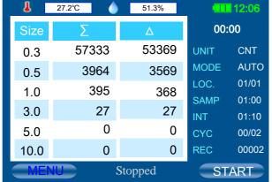
The sampling stops automatically when all cycles have finished.
