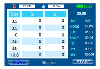
In this mode, P611 accumulates and updates the concentration data every 6 seconds. The result is only shown in /CF, /M3, or /L. Once it starts sampling, it will not stop automatically. Please press **STOP** to finish sampling. The data are recorded every 6 seconds.
