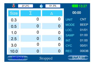
In this mode, P611 will beep according to the alarm setting of each channel. The number for alarm setting can only be set in  $\sum$  cumulative count (CNT). When none of the channels is selected, the setting for CH 1 will be activated. (It beeps when it reaches CH 1 alarm setting). If multiple channels are selected, it beeps when any of the selected channels reaches the alarm setting. Minimum sampling time is 6 seconds. Other functions are the same as Auto mode.
