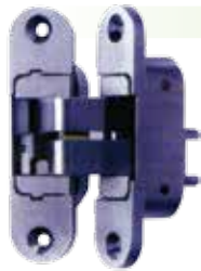
ST-C118 Suitable for doors from 600 to 1000mm width and up to 2700mm height with a minimal door thickness of 40mm. Load capacity 80kgs. *We recommend always 3 hinges installed!
