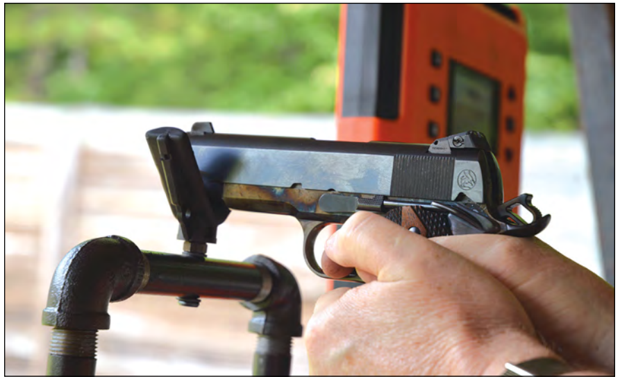
A LabRadar chronograph was used to measure muzzle velocity when testing the Commander Heritage .45 ACP.
