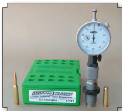
A Redding Instant Indicator-Case Comparator is an excellent tool for adjusting a sizing die to obtain correct headspace and determine datum length.
