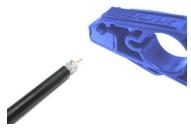
Fold the braided shield back onto the outer jacket.
