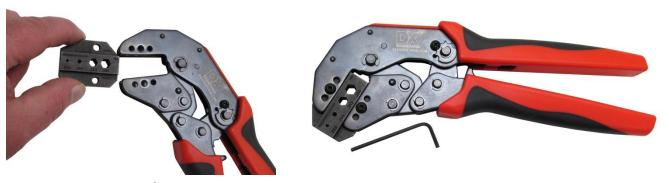
When installing the Powerpole<sup>®</sup> Die Set, use the supplied longer screw and Nyloc Nut and washer to allow for the addition of the Powerpole<sup>®</sup> crimp connector holder.
