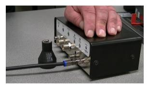
Reverse the process to remove an F Connector from your unit.
