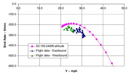
Figure 17. Author's crude flight test comparison with built up Sport 2 data
