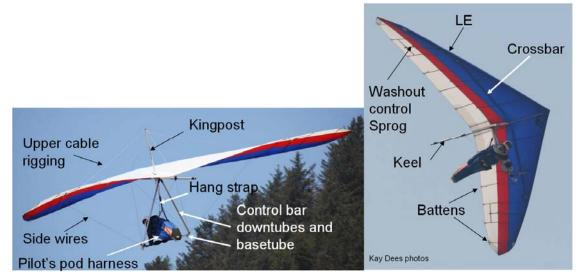
Figure 3. Flex-wing hang glider parts
