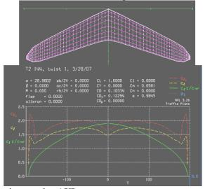
Figure 12. T2 Induced drag estimate using AVL.
