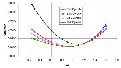
Figure 14. Adjusted profile drag estimates
