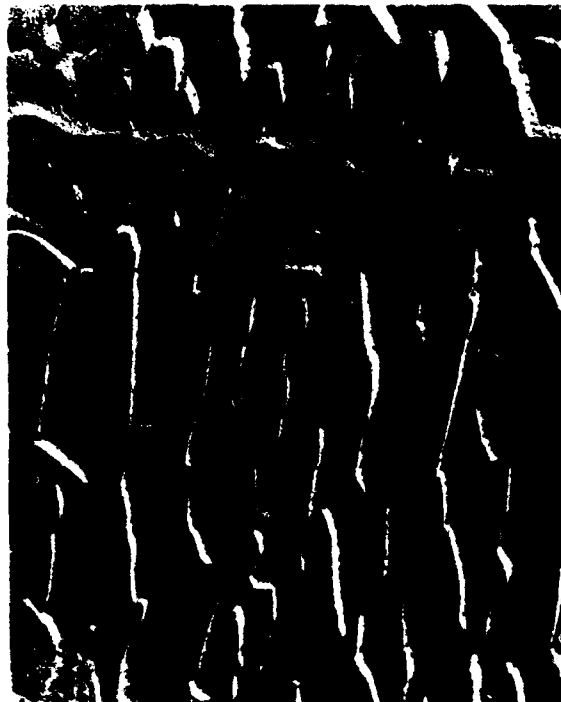
Figure 14. Electron replica photography showing increasing amounts of precipitates with Ti contents in Fe-9Ni-9Co-Ti alloys aged at 800°C for 17 hr. Mag. 10,000X.
