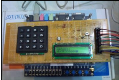
Fig. 7. I/O interface circuit on donut board with working LCD display
