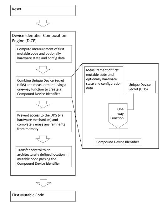
manufacturer in any way that is consistent with this specification. Any revision c of the measured components results in a different value for the CDI.
