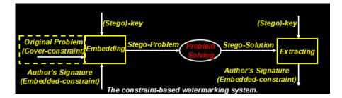
Fig. 7. Digital watermarking for IP protection as a steganography system [11].
