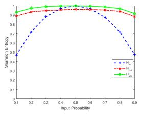
PUF is combined with XOR. This indicates a cost effective way to convert data from a poor entropy source to high entropy bit-stream.
