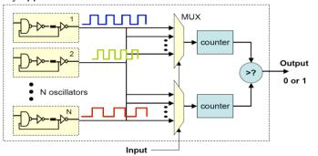
Fig. 3. The architecture of ring oscillator PUF [6].
