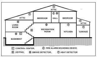
At least one smoke detector should be installed directly outside each sleeping area. If there is more than one floor, additional smoke detectors should be installed on each level, including the basement. The living-area and basement smoke detectors should be installed near the stairway of the next upper level.
