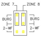
The GEM-P3200 can use conventional 12 VDC 4-wire smoke detectors. To use them, the select fire zone programming option and do not select 2-wire smoke detector programming option for the desired fire zone (refer to the GEM-P3200 Programming Instructions). Set JP7 to the position as shown, if zones 7 or 8 are to be used.
