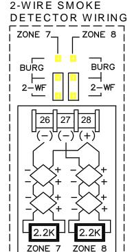
Two-wire smoke detectors can only be connected to zones 7 and 8. To use them, select fire zone programming option and select 2-wire smoke detector programming option for the desired fire zone 7 or 8 (refer to the GEM-P3200 Programming Instructions) and set JP7 to the position as shown. Connect the 2-wire smoke detectors as shown.
