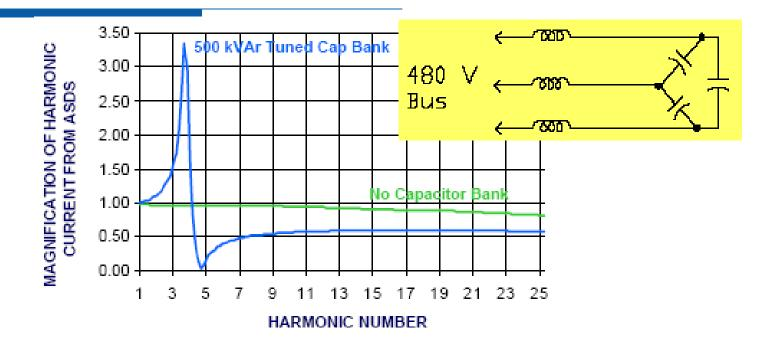
Reactors can be added to the PFCC bank to create a tuned filter
