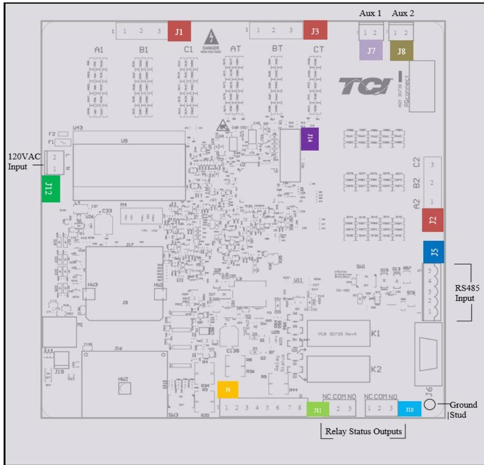
Figure 12: PQconnect Connections
