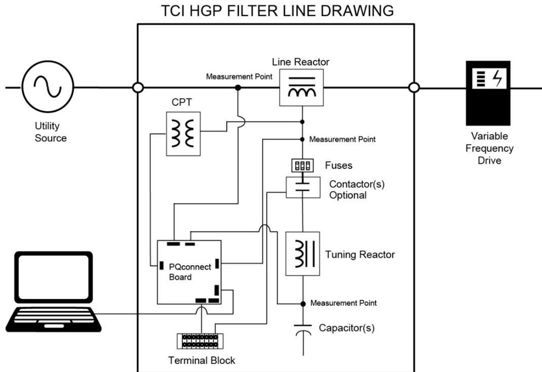
**Figure 4: HGP Filter with PQconnect Typical Connection Diagram**
