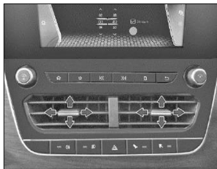
Centre Air Vents (Front)
