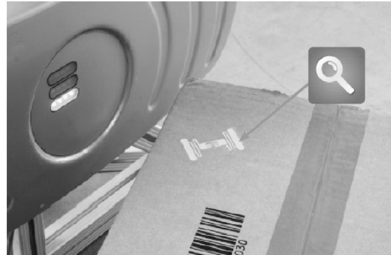
FIGURE 1-18 With an RFID tag, items can be tracked and monitored throughout the shipping process.
