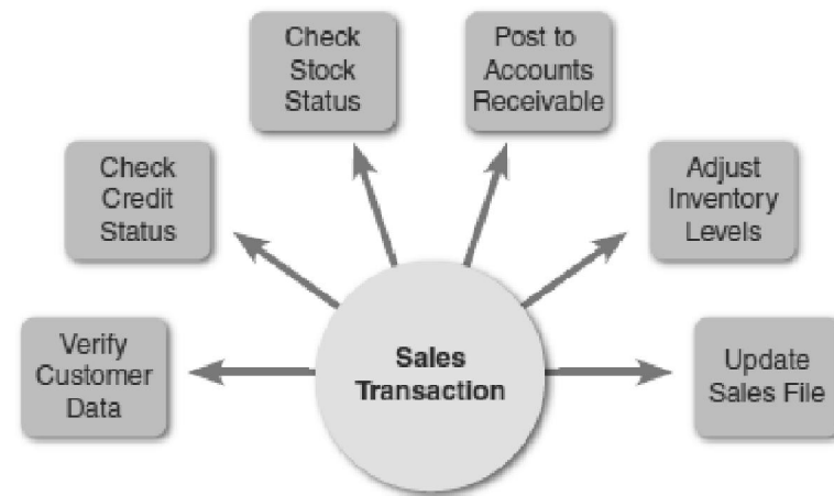
FIGURE 1-17 A single sales transaction consists of six separate tasks, which the TP system processes as a group.
