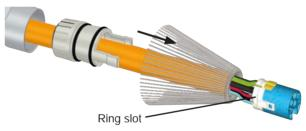
(4) Strip the shielding between the first and the second O-ring!
