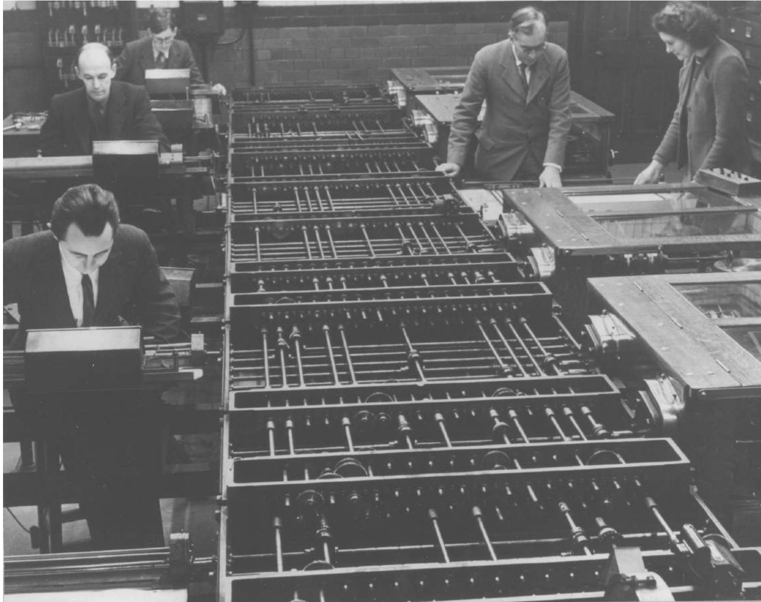
Douglas Hartree and Phyllis Nicolson attending the operation of the Differential Analyzer
