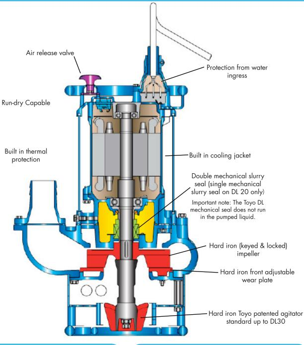
The Toyo patented agitator eliminates solids accumulating on the sump floor and can significantly reduce maintenance costs resulting from digging out sumps and downtime due to solids building up and choking off the suction of conventional pumps. It is because of the Toyo Agitator's patented blade that the highest efficiency in material mixing can be achieved.
