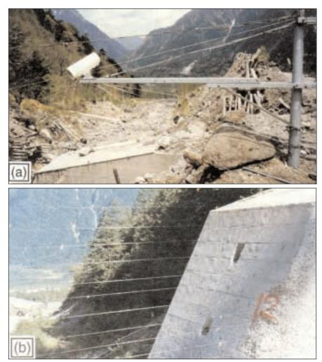
Figure 27. Examples of monitoring devices for debris flow warnings, (a) -a current gage and (b) a wire sensor system. (Photos from United Nations, 1996)
