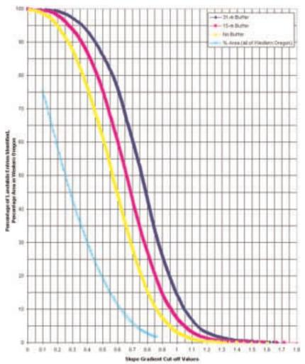
Figure 20. Percentage of landslides identified by various slope threshold selections. (Adapted from Hofmeister and Miller, in preparation)
