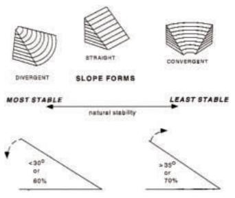
Figure 13. Schematic of divergent, straight, and convergent topography. (From Benda and others, 2000)
