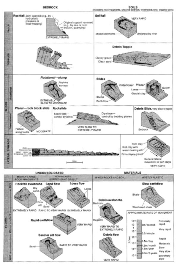
Figure 3. Landslide types. (From Ritter and others, 1995)
