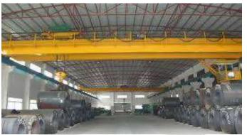
Fig. 1: Electric Overhead Travelling (EOT) crane
