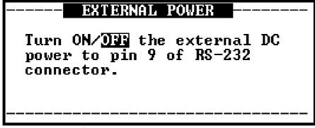
Figure 4-41 : External Power Setup
