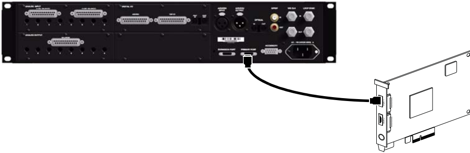
Figure 1. HD I/O connected to the DigiLink Mini Port 1 on an HD Native card
