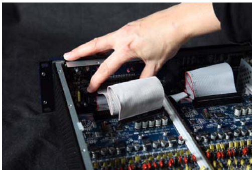
Connecting the 50-pin cable to the HD I/O chassis
