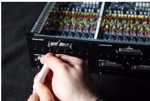
Removing the screws securing an I/O card
