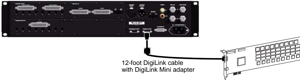
Figure 3. HD I/O connected to the DigiLink Port on a Pro Tools|HD Accel Core card (16-channel I/O system)
