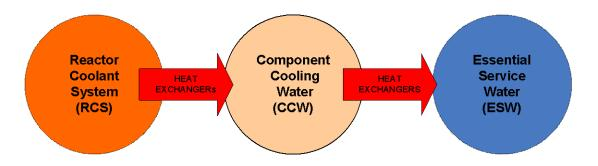
The **Essential Service Water System** (ESW) is designed to provide a source of cooling water to multiple heat exchangers required for the safe shutdown of the reactor following an event.
