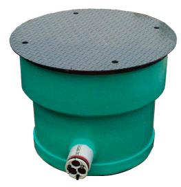
The MOV 300 series are specifically designed for fiber optic OSP underground applications. The MOV 330-WT is a watertight version of the popular handhole designed to provide a watertight environment for electronic components to prevent the infiltration of natural groundwater in the vault.
