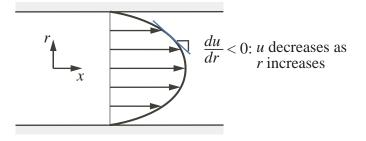
Since the pressure gradient is constant for fully-developed flow
