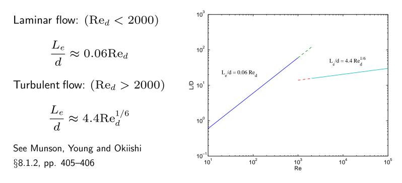
In most design calculations, the flow in straight sections is assumed to be fully developed. The entrance length correlations are used to check to see whether this is a good assumption.
