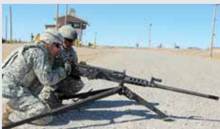
1AD Soldiers train on M205 Lightweight Tripod with a mounted M2A1 .50 Caliber Machine Gun at Fort Bliss, TX. The M205’s lightweight pintle allows greater weapon elevation and depression than the M3’s pintle.
