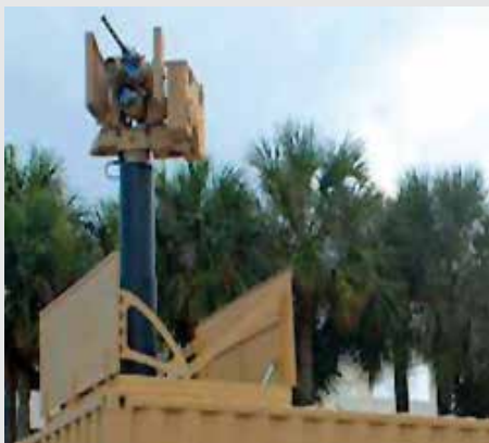
CROWS Containerized Weapon System increases options for integrated base defense in difficult to reach and remote locations.
