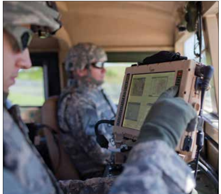
By allowing multiple software programs to utilize a single hardware solution inside the vehicle—rather than requiring individual hardware—the Mounted Family of Computer Systems also reduces size, weight, and power demands. (DRS Technologies, Inc.)
