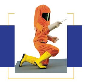
Arc suit is a specially designed protection garment used worldwide to effectively protect human life from electric flash. They are made from special **flame retardant fabric (FR)** complying to **IEC 61482-1 & IEC 61482-2** and tested as per **ASTM 1959**. They are classified a per HRC 1, HRC 2, HRC 3, HRC 4, based on ATPV values, as per **NFPA 70 E** values.
