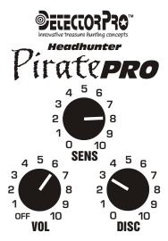
**HEADHUNTER PiratePRO** model has three controls for the micro-encapsulated circuitry located in one sealed earcup of the headphones. Batteries are found in the other earcup and are user accessible.
