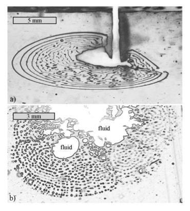
Figure 2. Geometry of healed cracks depending on the injected fluid. a) Healed crack originally filled with liquid epoxy glue showing the concentric channels of fluid trapped during the healing process. Some fluid is still trapped in the open portion of the crack. b) Healed crack originally filled with motor oil. With time the channels of trapped fluid become unstable and fragment into single spherical inclusions. Finally a concentric network of fluid inclusions pervades the healed region.
