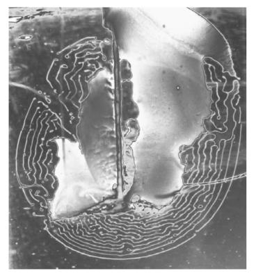
Figure 5. Fluid inclusion pattern of healed cracks.
