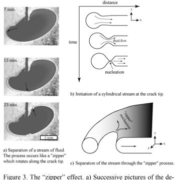
tachment of a cylindrical fluid inclusion at the crack tip in an epoxy-filled crack. b) Sketch of the initiation of a cylinder at the crack tip. c) Then a channel of fluid separates. While the pressure gradient is radial in the open portion of the crack, it becomes tangential near the channel. The process is driven by surface tension and elastic energy released by the walls of the crack. The channels detach like a " zipper" from the open part of the crack.
