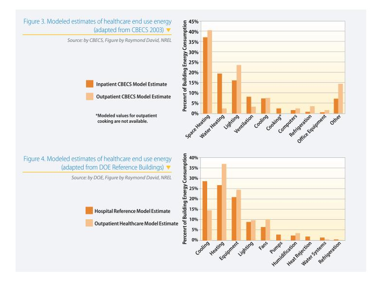
In particular, heating, cooling, lighting, fans/ventilation, and plug/ process equipment are suspected to consume greater energy than other end uses in a typical healthcare facility. These general indications can be combined with site-specific needs to determine where first efforts should be spent in conducting feasibility assessments and requesting quotes for metering products and services.
