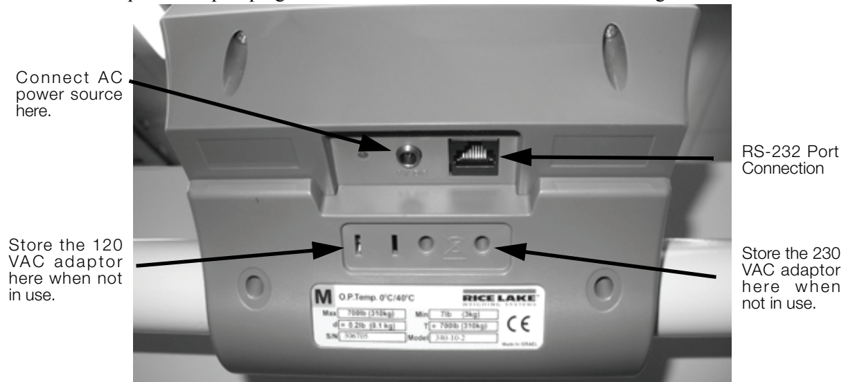
Figure 0-2. AC Power and RS-232 Connection Site
