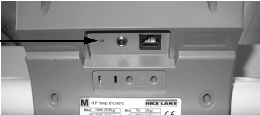
Figure 1-2. LED Light Location
