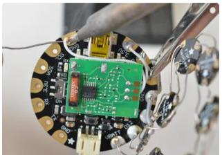
Wire up and solder the sensor to the FLORA main board according to the circuit diagram on the previous page.
