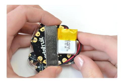
Stick the metal bar of the magnetic pin back on the back of the board, and use another piece of double-stick tape to attach the small lipoly battery right next to it.
