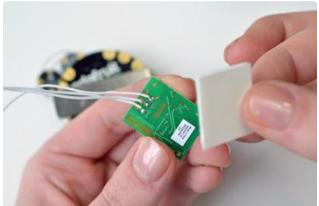
Solder three small wires to the Polar heart rate receiver, and stick it to the FLORA main board with a piece of double-stick tape or foam.
