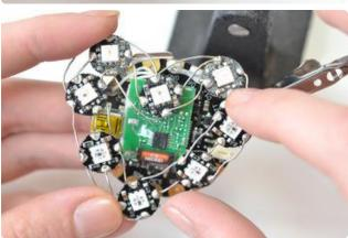
Place a piece of tape over the sensor to prevent the pixel display from shorting its contacts. Lay out and solder together your heart-shaped pixel display according to the circuit diagram on the previous page, then solder the heart shape to VBATT, GND, and D12 on the FLORA main board.
