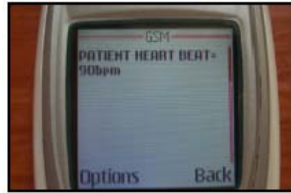
Figure 8. SMS Testing from GSM Modem to Cell phone. Alert message appears on mobile phone screen.
