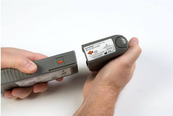
Figure 9 Inserting battery into clip
