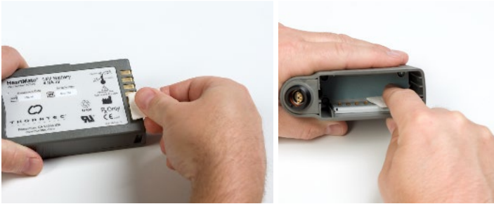
Figure 11 Cleaning metal battery contacts and contacts inside of battery clip
