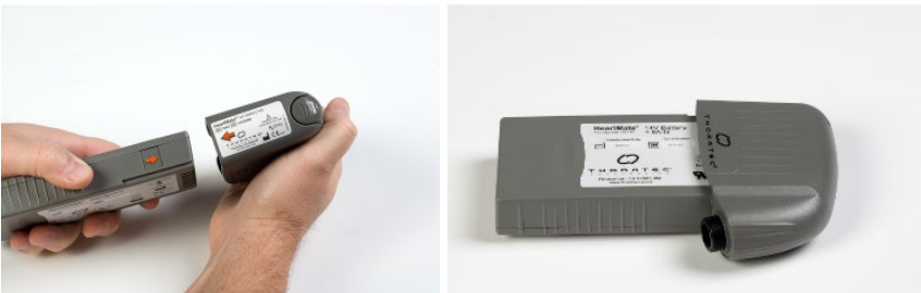
Figure 6 Inserting HeartMate 14 volt Li-Ion battery into 14 volt battery clip
