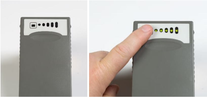
Figure 5 Battery fuel gauge (note battery symbol)
