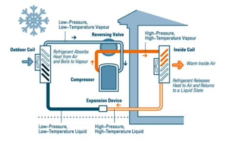
Figure 1. The components and operation of heating cycle (WayneWhiteCoop, 2012)
