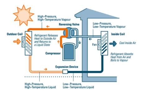
Figure 2. The components and operation of cooling cycle (WayneWhiteCoop, 2012)
