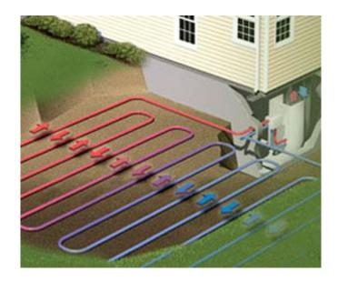
Figure 4. Illustration of a ground-source heat pump (Glynns, 2012)
