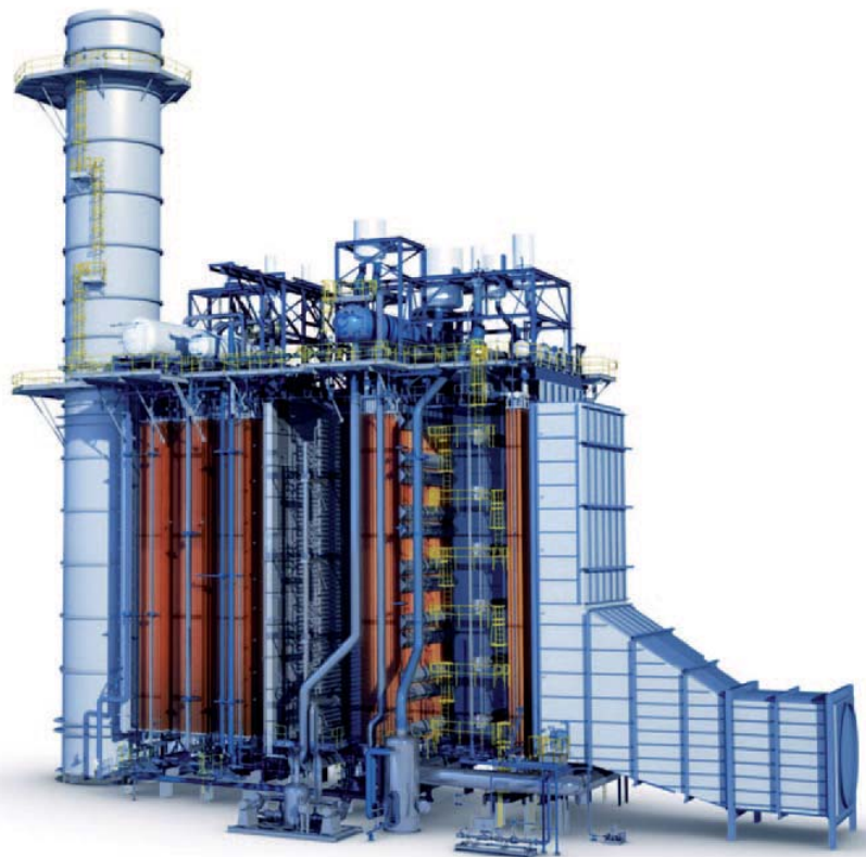
HRSG – Triple pressure reheat design with supplementary firing and emission control equipment for CO, VOC and NOx
