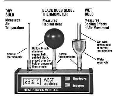
Heat stress monitors currently available calculate WBGT automatically. The equipment required and the method of measuring WBGT can be found in the ACGIH booklet *TLVs® and BEIs®: Threshold Limit Values...Biological Exposure Indices.* The booklet also outlines permissible exposure limits for heat stress. Older instruments, however, require calculation by the operator.
